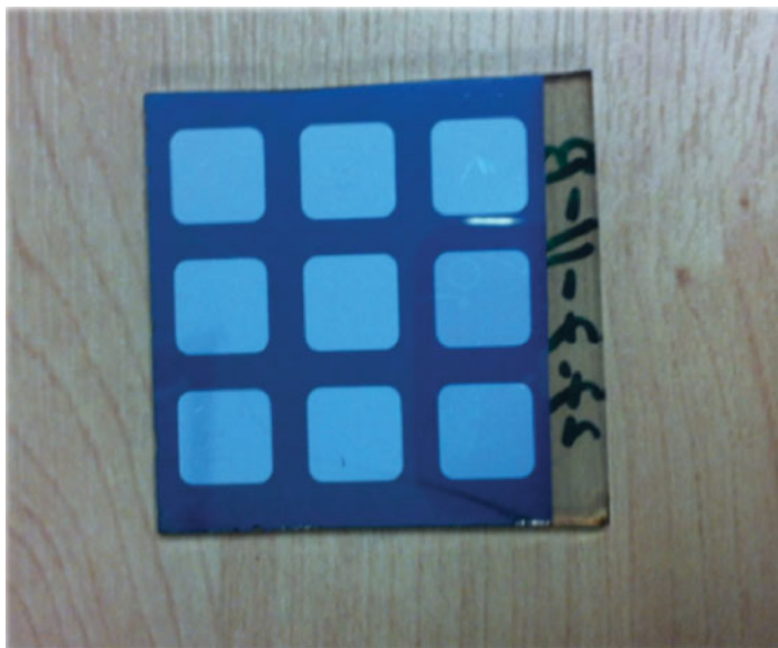
Figure 19. P-I-N device with 3 \times 3 contact grid.
